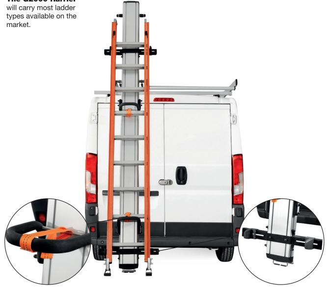
The new version of the G2000 Harrier has added features to further improve the safe transport of ladders when the vehicle is moving.
