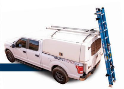
With the G2000 series, health risks to the back and shoulders are dramatically reduced when loading / unloading long and heavy ladders because the operations are assisted by a hydraulic assistance system reducing the effort required to a minimum.
