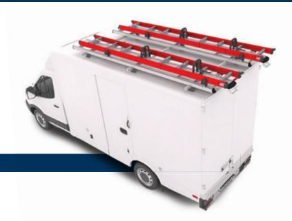
Maximize rooftops utility with 2 x G2000 Harrier ladder racks that allow loading up to 2 x ladders by stacking and up to 132 lbs. on each ladder rack.
